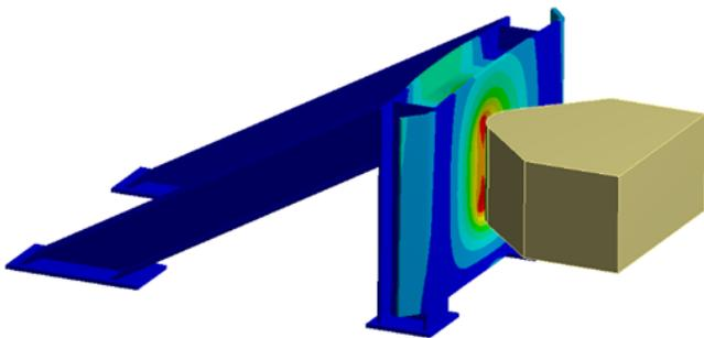
**Figure 1.** Imported Pressure distribution from CFD
