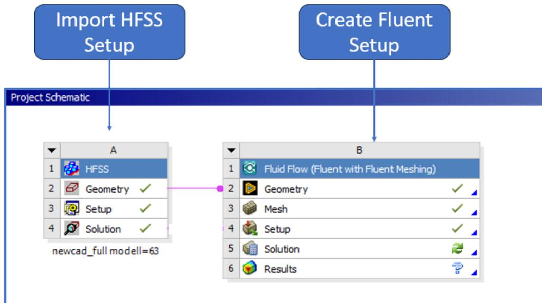
**Figure 3.** Workbench HFSS - Fluent Coupling
