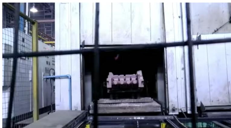
**Figure 2.** Industrial Microwave Dryer for Metal Casting.
