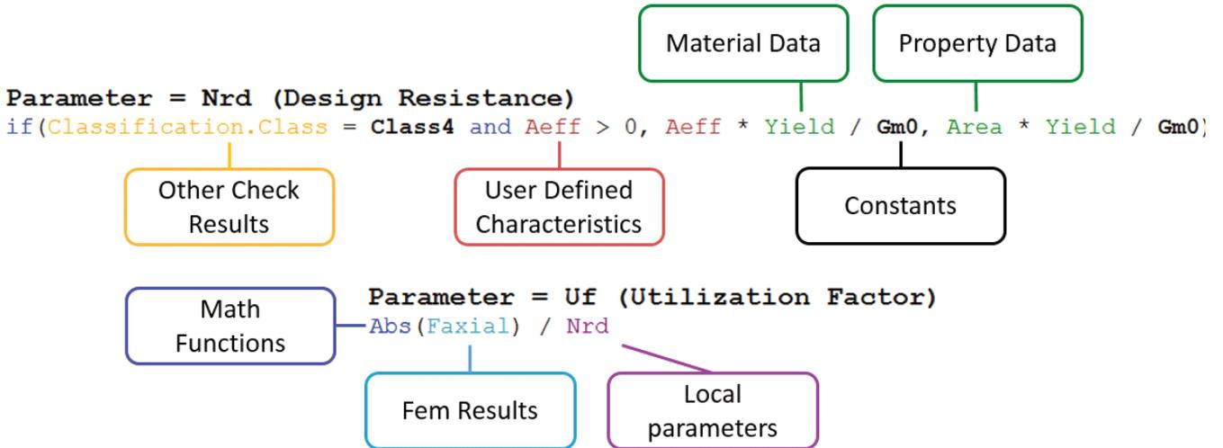
The following example demonstrates a verification of bolted connections. The Axial Force of bolts is compared with the bolt design resistance:
