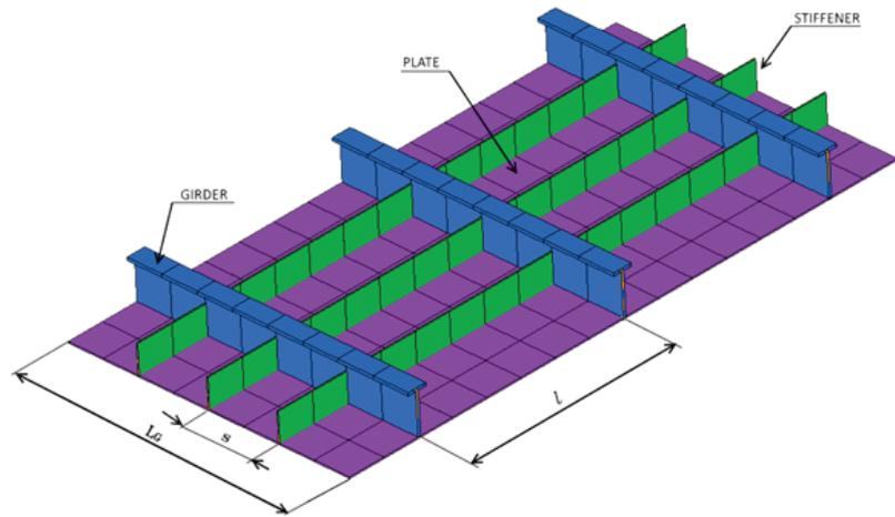
In the figure below panels, simple stiffeners (marked in blue) and girders or stiffeners which support also other stiffeners (marked in red) are plotted.
