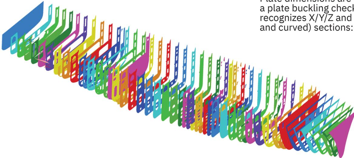
The recognition is based on the mesh connectivity and can be performed on any structure using plate (*shell*) elements:
