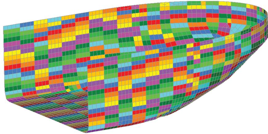
**Stiffened Panel Finder** — recognizes sections, panels, plates, stiffeners and girders and their dimensions automatically. This tool is an advanced version of the Panel Finder.
