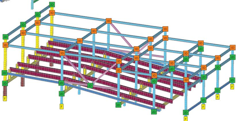
The deflection of members is one of the checks that should be performed for serviceability limit state design. With the help of **Beam Member Finder** tool SDC Verifier automatically recognizes beam member lengths:
