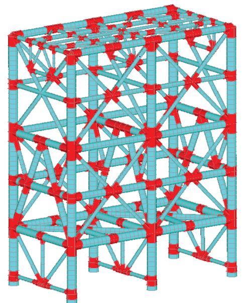
**SDC Verifier** calculates Brace classification (*depends on the load pattern*) for each load situation automatically, which significantly speeds-up the verification process.
