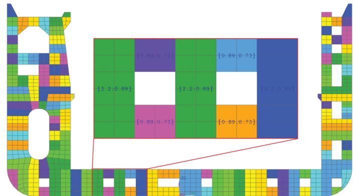
The results can be presented over sections (frames/longitudinals/decks) and results which are above the limit are highlighted with red:
