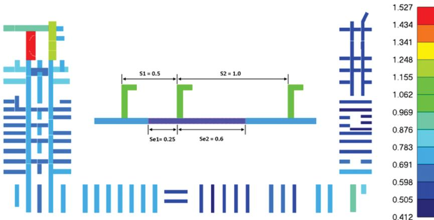
**Effective Width** — calculates the plate effective width for every load situation. The Effective width is used in the stiffener buckling check according to DNV-RP-C201 2010
