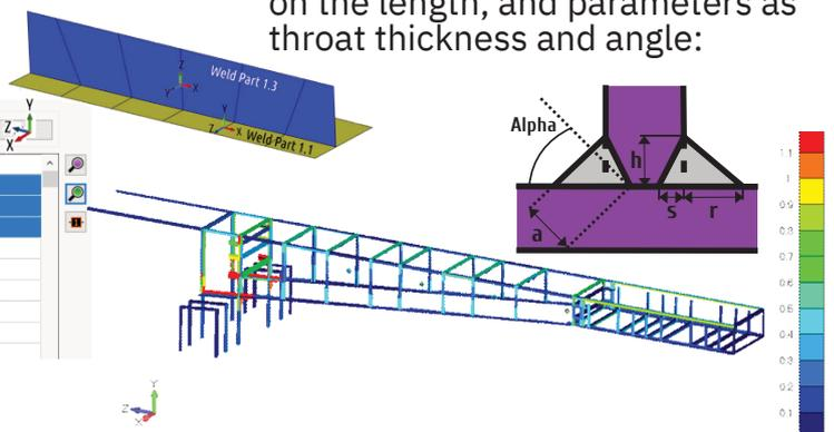
The notch group classification or fatigue strength of the welds depends on the quality and the stress direction, along the weld (X), perpendicular to the weld (Y) and the shear (XY). Stresses are converted into weld direction automatically by the weld finder.
