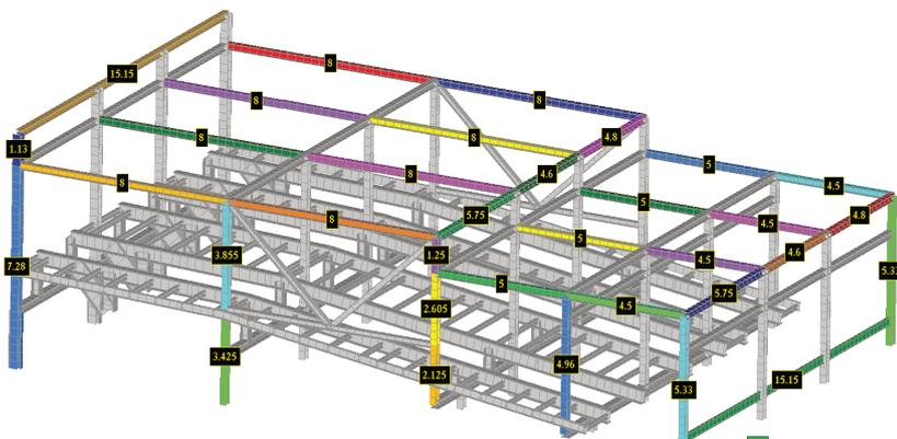
**Beam Member Finder** tool recognizes beam members (*buckling*) lengths automatically for 3 directions (*Y, Z and torsional*)
